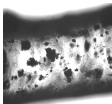
Figure 3. Morphology of 5 wt% PANI-LES in PP based materials/matrix polymer blends with twin screw blend, as revealed by bright field reflected light optical microscopy
