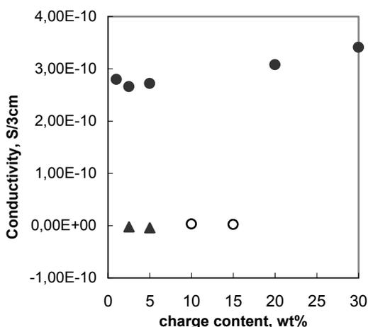
Figure 2. Electric conductivity of conductive materials/matrix polymer blends with twin screw blend, as revealed by bright field reflected light optical extruder: (●) PANI-LES in PP, (▲) PANI-LES in LDPE, (○) graphite in PP
