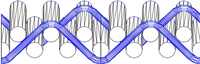
Figure 11. Virtual model of a woven fabric with a single warp thread system piled up
