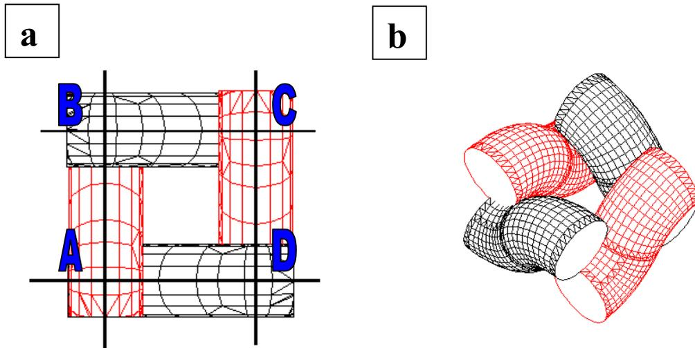
**Figure 1.** Model of a woven fabric of square structure (i.e. of equal warp & weft structure, which means of equal warp & weft sets, thread diameters, and material), double-system resistance surface, with non-deformable threads of circular cross-sections, and plain weave: a) perpendicular projection of one woven fabric element, b) view of a skew projection of this element.
