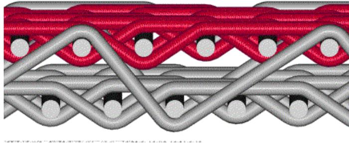
**Figure 13.** Double-woven fabric with layers joined by stitching from back to face with controlled channel dislocation in the layers.
