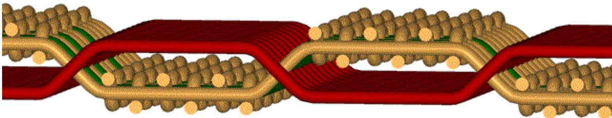
**Figure 14.** Virtual model of a double-layer woven fabric joined by the layer exchange method [7]
