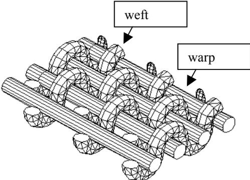
**Figure 4.** Model of the woven fabric presented in Figure 1 after changing the previously existing phase in a limiting structure phase with a weft single-system resistance surface.
