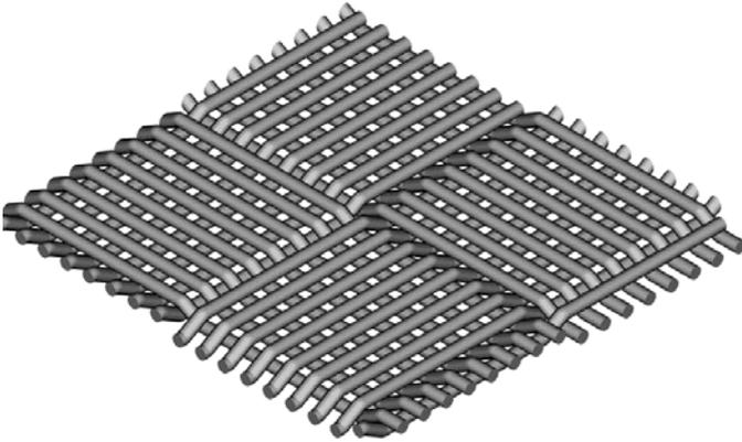
Figure 2. Hopsack weave with  $R_o = R_w = 16$ ,  $p_o = p_w = 2$ , [8]
