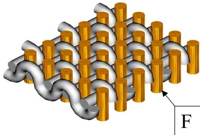
**Figure 8.** Virtual model of a woven fabric with an inter-thread channel filler (W).
