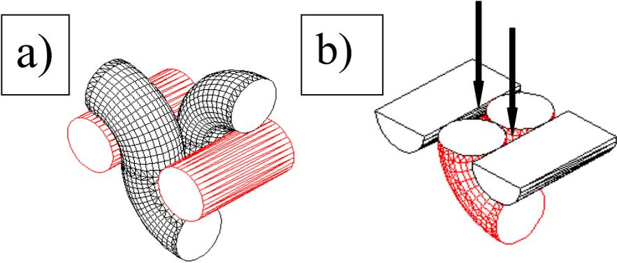
**Figure 5.** Virtual model of the woven fabric presented in Figure 1 after changing its phase in the limiting structure phase and increasing the weft thread set up to the limiting value  $Z_w = 100\%$ : a) view of the skew projection of a weave modulus, b) view of the same modulus but cut in the plane of half the diameter of the warp threads.
