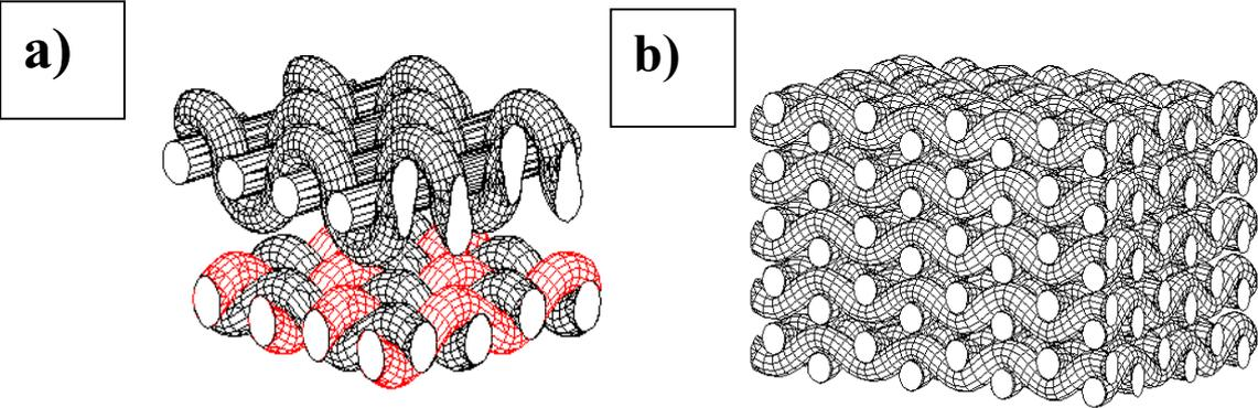
Figure 12. A simple piling-up of two woven fabric systems – a woven fabric barrier: a) a double-layer barrier from woven fabrics with different weave moduli, b) a five-layer barrier from structural identical woven fabrics.
