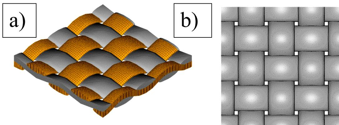
**Figure 7.** Virtual model of a square woven fabric with a double-system surface resistance: a) view of the skew projection, b) view of the perpendicular projection [6].
