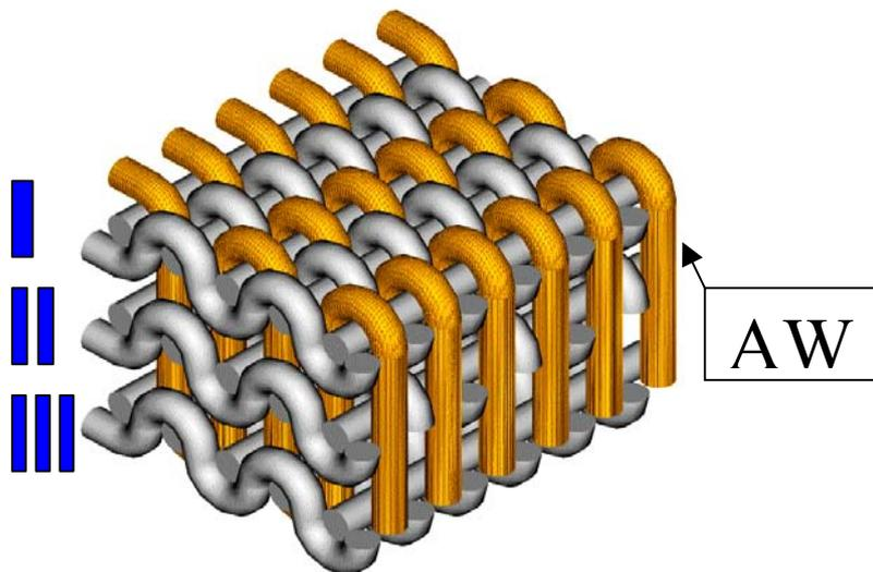
**Figure 9.** Virtual model of a ternary woven fabric with layers I, II, and III joined by an additional warp (OD).
