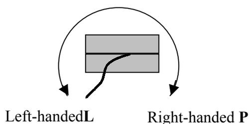
Figure 3. Fibre turning directions
