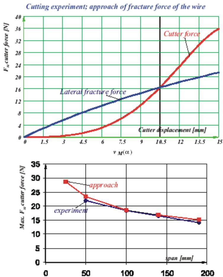
Figure 7. Determination of critical cutting force and comparison with experiment at different spans
