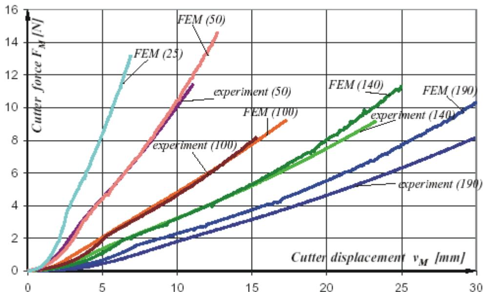
Figure 2. Weaving wire - comparison experiment-FEM (spans 190,140,100,50,25 mm)
