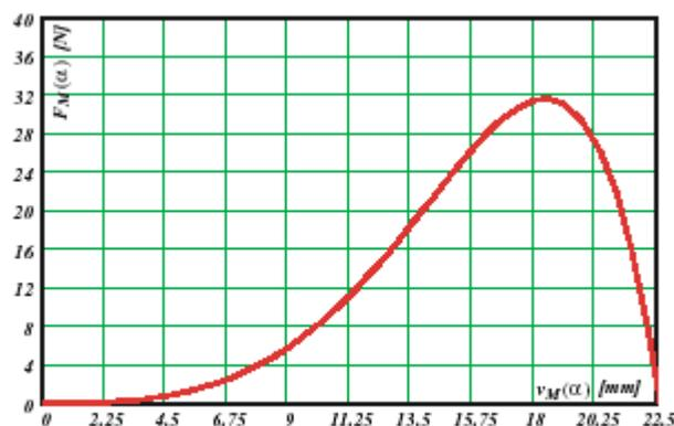
*Cutter force -fracture:  $F_{Mmax} = 31.5 \text{ N}$  at  $\alpha = 11.2^\circ$  resp.  $v_M = 18.5 \text{ mm}$
