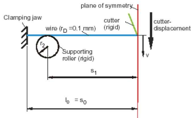
Figure 1. Principle model and cutter geometry
