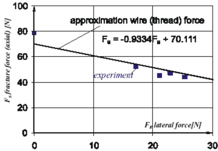
Figure 6. Correlation critical cutting force: axial and lateral stress
