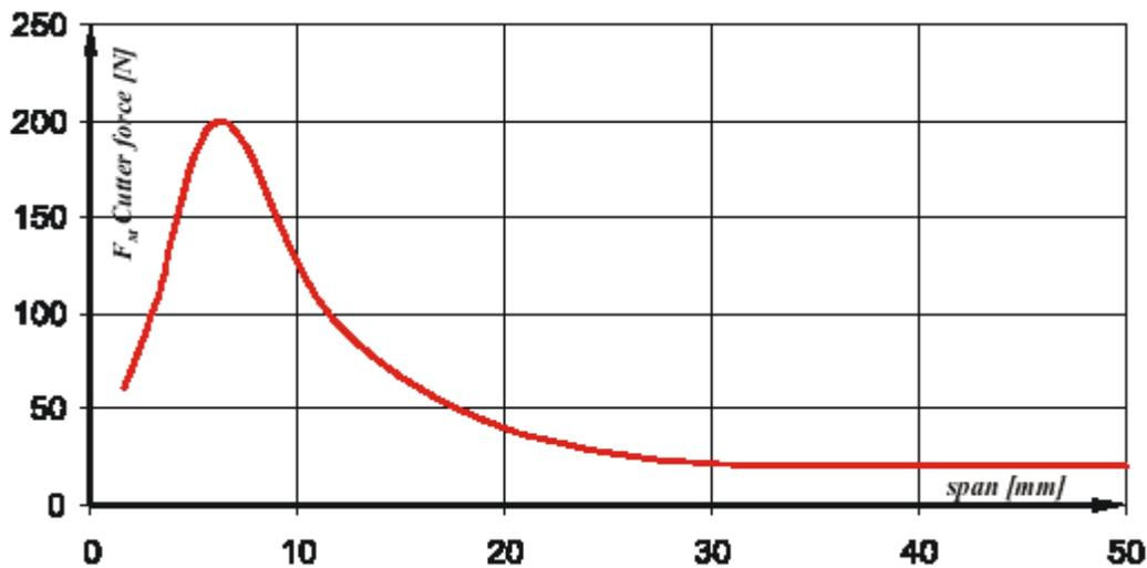
Figure 4. Cutting force in dependence of span
