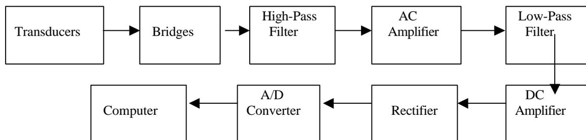
**Figure 4:** Schematic of the electronic components used in the system
