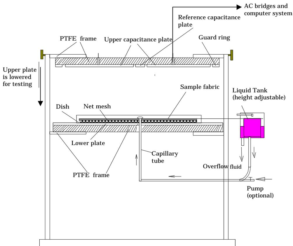
Figure 1: Schematic Diagram of the Measuring Instrument
