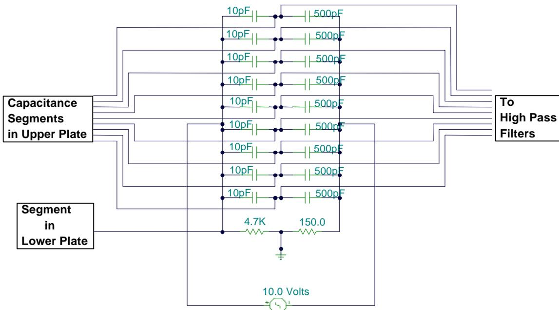
**Figure 3:** Schematic of the A.C. bridges set-up used in the system
