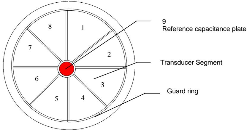
**Figure 2:** Alignment of transducer segments in the upper plate of the capacitance system
