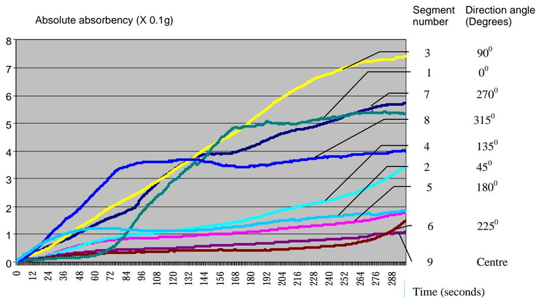
**Figure 5(b)** Example of dynamic liquid absorption measurements vs. time (Cartesian system)
