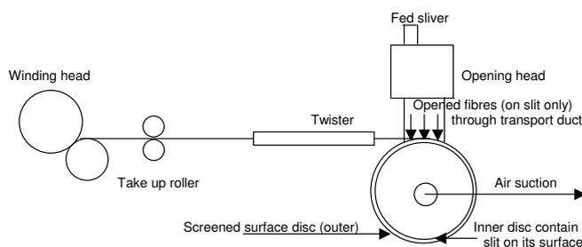
Figure 1b. Details of the disc and location of slit angle
