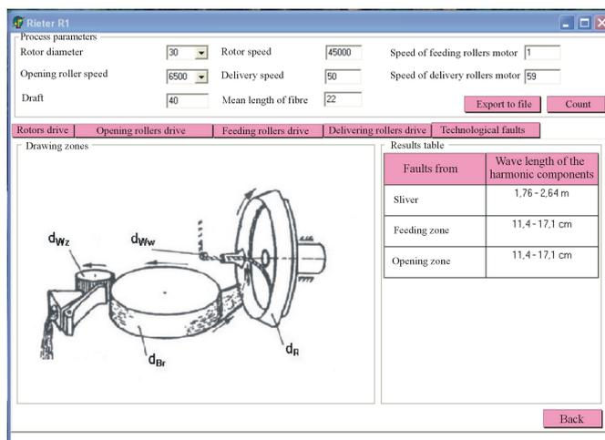
Figure 2. Sample programme window - technological faults.
