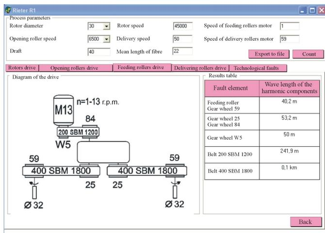
Figure 1. Sample programme window - feeding rollers drive.
