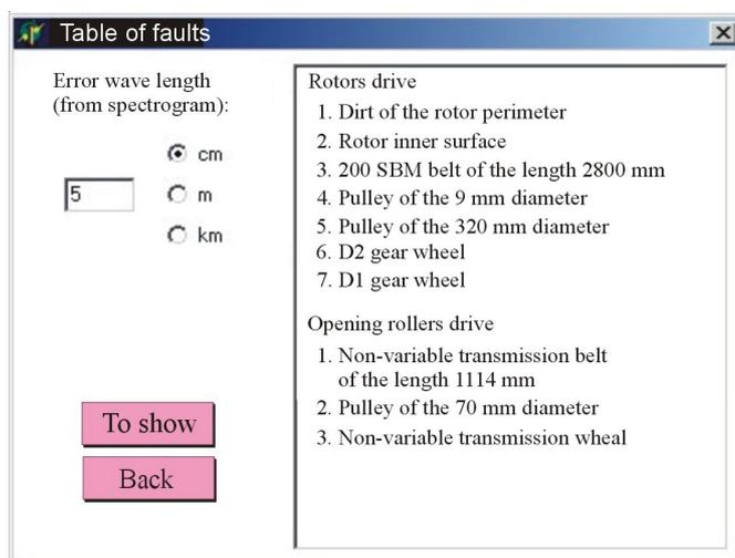
Figure 3. Table of faults, result screen.
