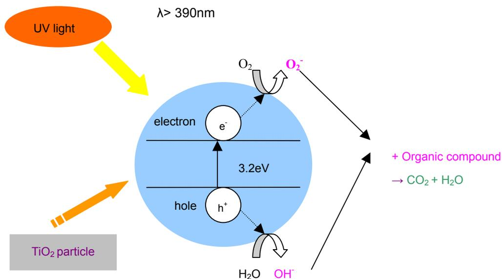
**Figure 2.** Photocatalysis mechanism of titanium dioxide
