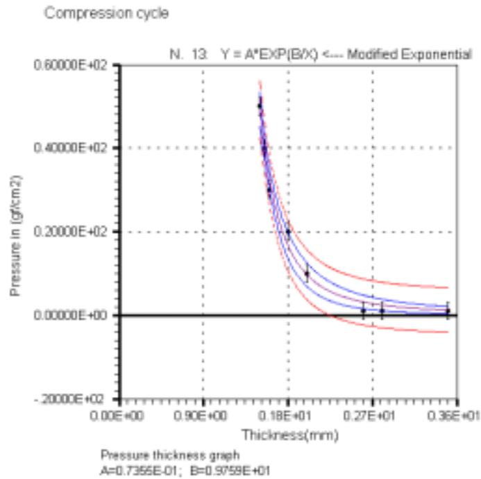
Figure 1. Pressure-thickness curve – compression cycle
