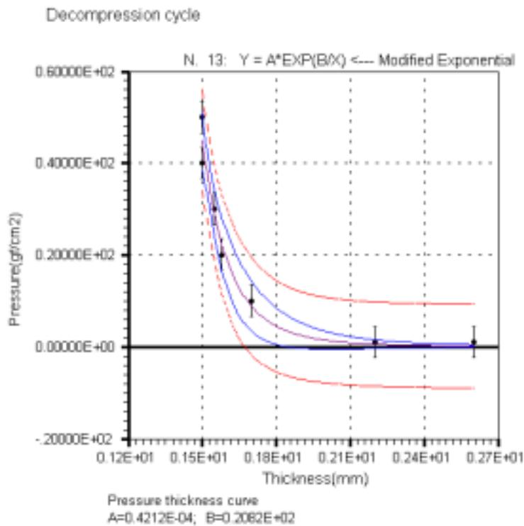
Figure 2. Pressure-thickness curve – decompression cycle
