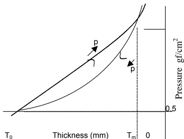
**Figure 3.** Pressure-thickness evaluation
