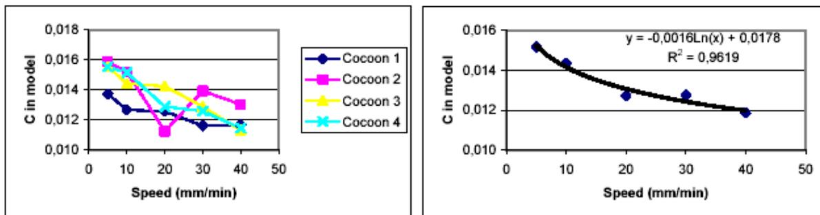
Figure 11. Influence of testing speed on parameter C in extended Maxwell model
