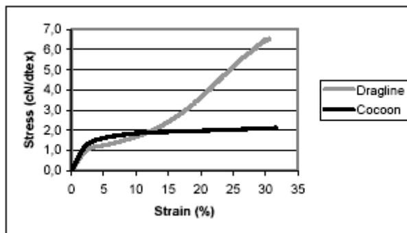
**Figure 1.** Stress-strain behaviour of cocoon and dragline spider silk of *A. diadematus*
