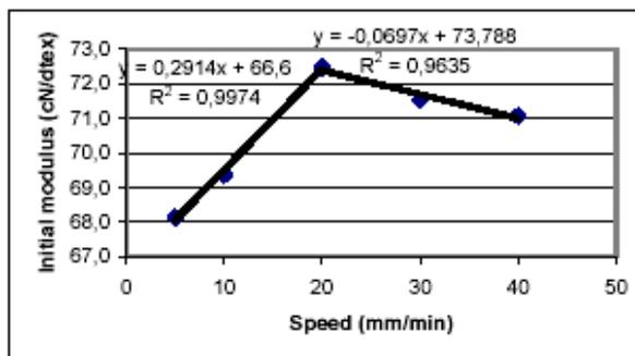
Figure 7. Relationship between initial modulus and speed
