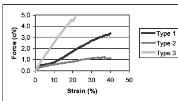
Figure 8. The three types of stress-strain curves occurring for dragline silk
