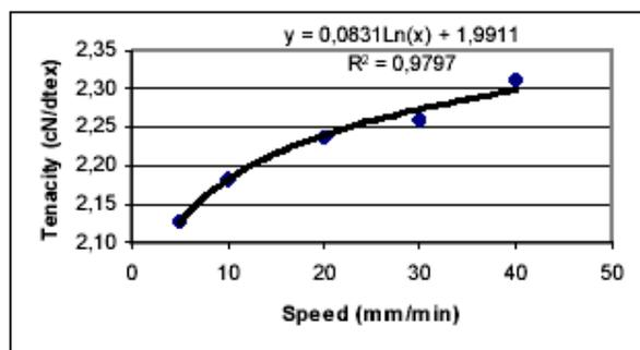
Figure 6. Logarithmic increase of tenacity with speed
