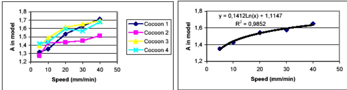
Figure 9. Influence of testing speed on parameter A in extended Maxwell model
