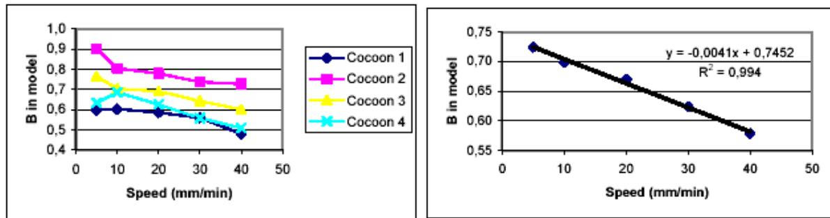
Figure 10. Influence of testing speed on parameter B in extended Maxwell model
