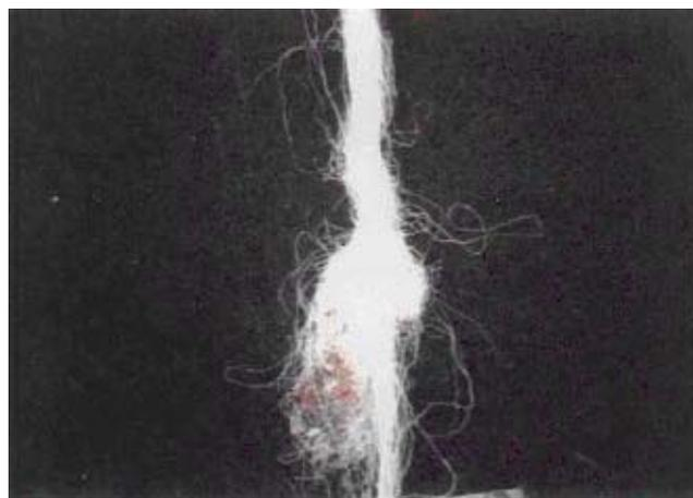
**Figure 3.** Broken end with seed coat embedded end
