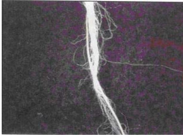
**Figure 1.** Broken end with foreign material embedded end
