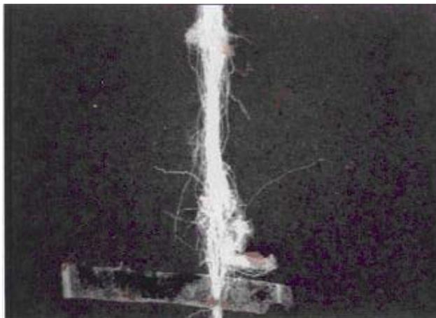
**Figure 4.** Broken end with trash particle embedded end
