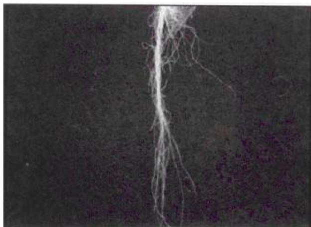
**Figure 5.** Broken end with tapered end
