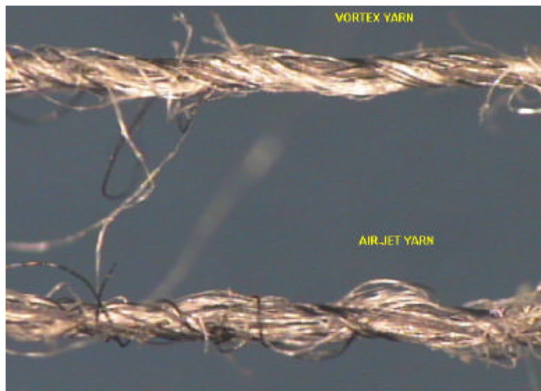
Figure 4. Vortex spun yarn versus air-jet spun yarn (28's Ne, 30/60 PES/Co)
