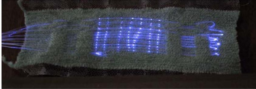
**Figure 6.** Fabric woven from steel (warp) and Trevira CS (weft) with 0.025mm notched 0.5mm PMMA POF weft floatings
