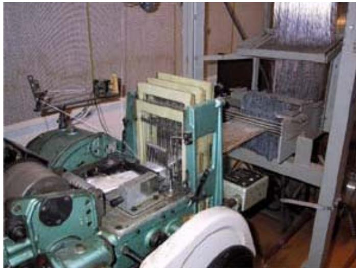
**Figure 3.** Narrow fabric weaving unit for POF fabric sample preparation in TUT
