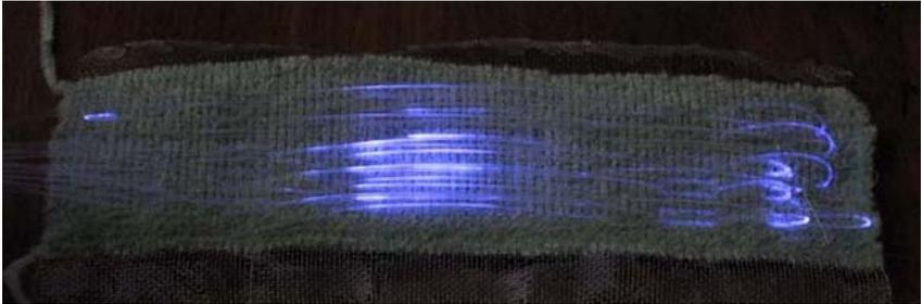
**Figure 5.** Fabric woven from steel (warp) and Trevira CS (weft) with Stoll abrasion treated 0.5mm PMMA POF weft floatings.
