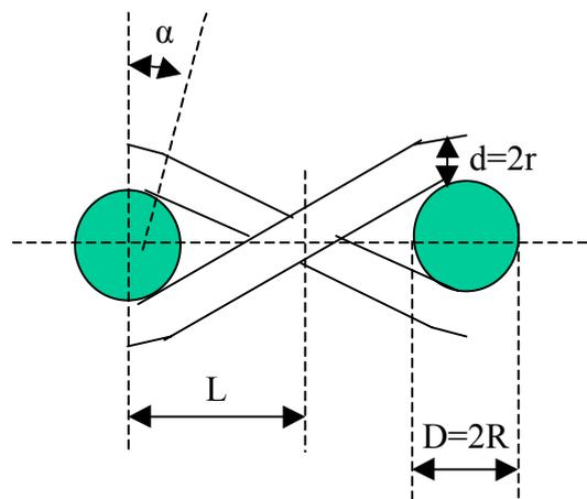
Figure 1. Schematic structure of a woven fabric
