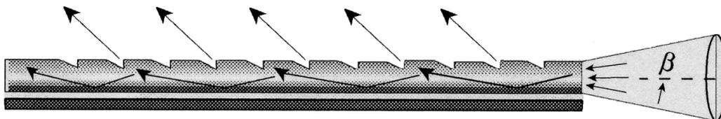
Figure 2. Optic fibre with dints
