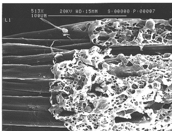
**Figure 1.** SEM micrograph of linen of type 1 laser treated
