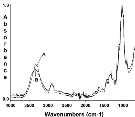
**Figure 5.** FTIR-ATR spectra of linen of type 3: A) untreated, B) laser treated
