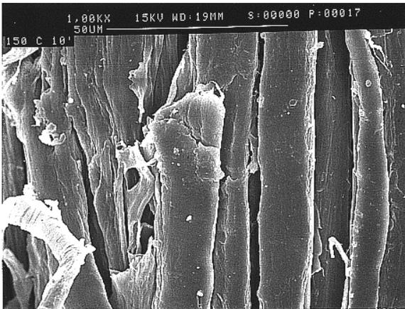
**Figure 9.** SEM micrograph of linen of type 3 after heat treatment at 150°C for 10 min
