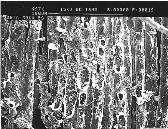
**Figure 8.** SEM micrograph of linen of type 3 after electron beam treatment
