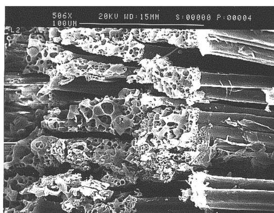
**Figure 2.** SEM micrograph of linen of type 2 laser treated
