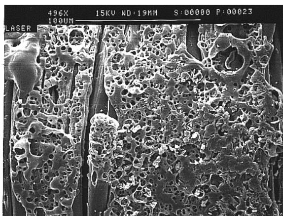
**Figure 4.** SEM micrograph of linen of type 3 laser treated
