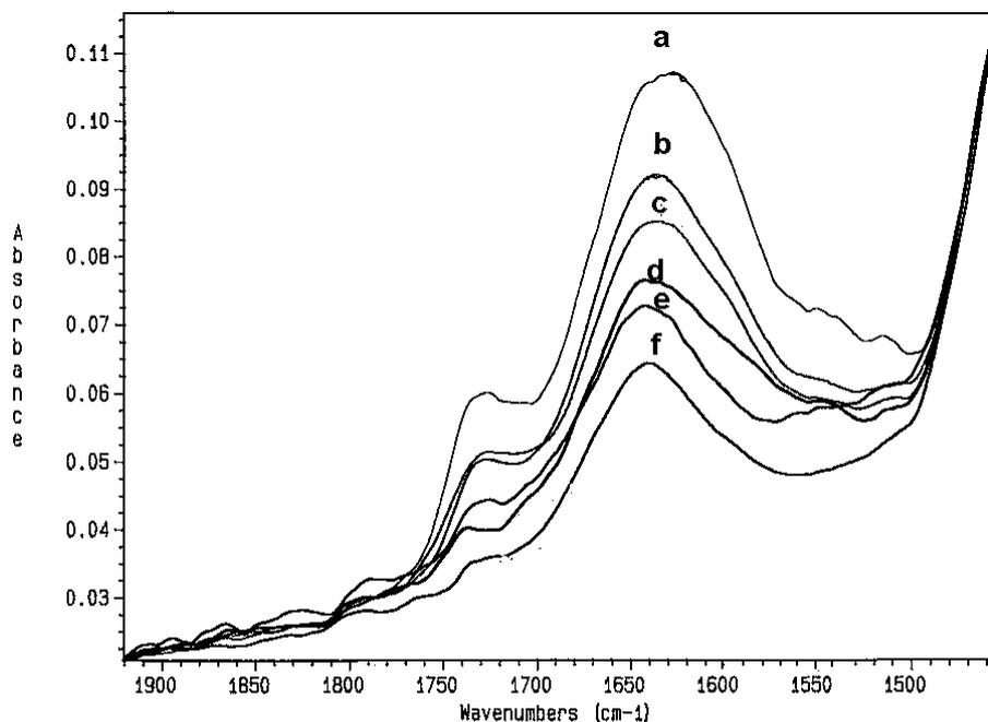
**Figure 3.** FTIR-ATR spectra of six linen samples: a) raw linen of type 2, b) linen of type 2 laser treated light, c) linen of type 2 laser treated darkened, d) linen of type 2 bleached, e) linen of type 1 laser treated light, f) linen of type 1 laser treated darkened
