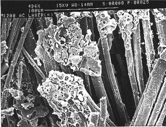
**Figure 6.** SEM micrograph of linen of type 4 laser treated
