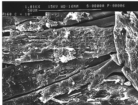
**Figure 10.** SEM micrograph of linen of type 3 after heat treatment at 160°C for 10 min
