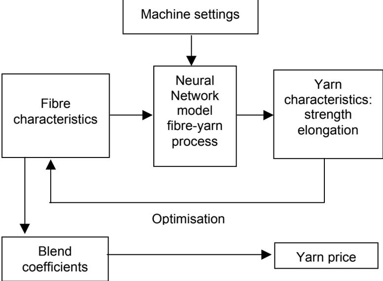
Figure 1: Fibre-yarn model based on fibre characteristics
