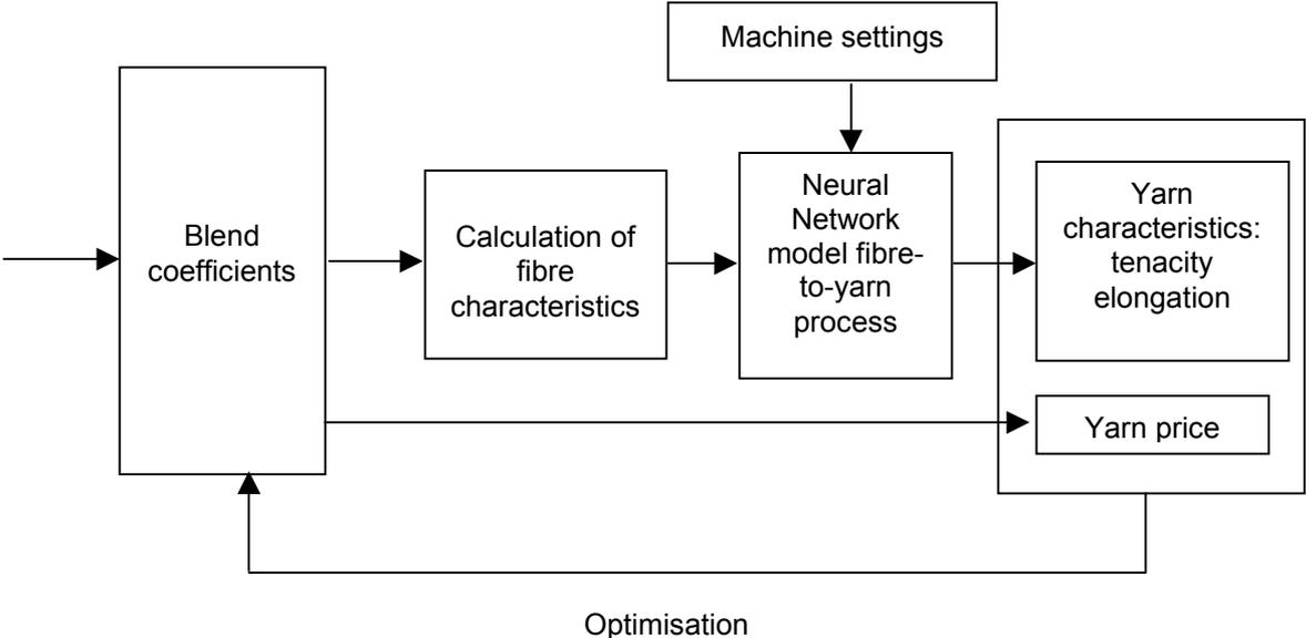
Figure 2: Fibre-to-yarn model based on blend coefficients.
