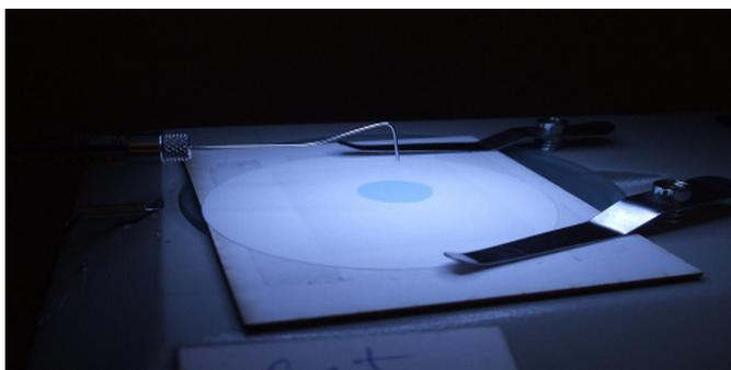
Figure 5. The needle and the sample positioned on microscope stage.
