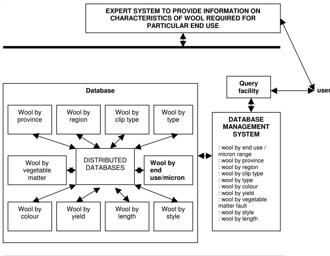
Figure 3. Architecture of wool utilization expert system
