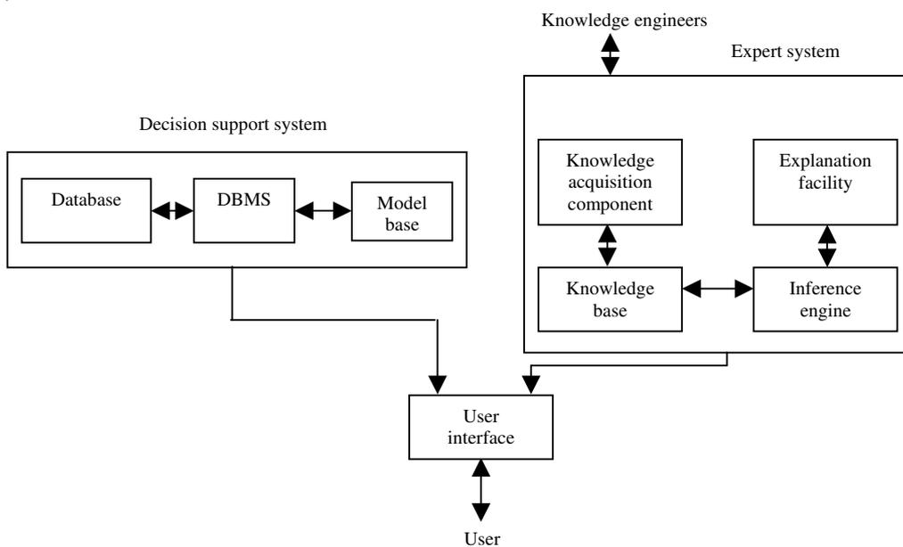
Figure 1. Architecture of DSS for wool classification and grading.
